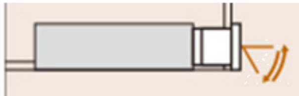
Horizontal louver 0~60°, 7 angle setting
